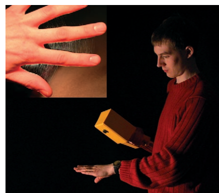
Figure 36. Handheld device for the electrospinning of wound dressings. Inset: PEO fibers electrospun from aqueous solution onto a hand.
